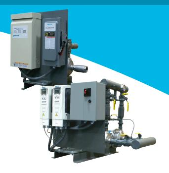
The AquaBoost VS is available in both one and two pump packages. Simplex capacities range from 20 to 110 GPM at a boost of up to 55 psig. Duplex capacities are up to 220 GPM.
