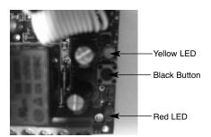
Place the control board back into the remote receiver cover and reinstall the cover by aligning the four plastic posts on the base with the four holes in the cover. Make sure the white wire is properly inserted into the cover cutout. Gently snap the cover and base together.
