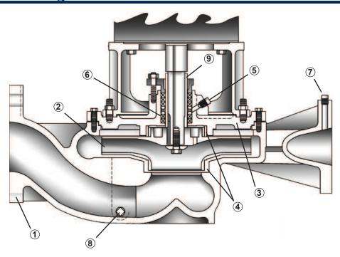
**1.Casing** - Flanged suction and discharge on common centerline. Integral one-piece unit suitable for in-line or pedestal mounting. Designed for working pressures up to 350 PSI with ½" corrosion
